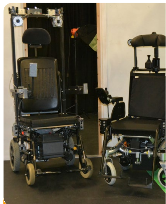
Test and trial chairs: The development of assistive powered wheelchair technology requires an academic test platform (left) to develop and test algorithms and sensors, which when functional are then transferred to the clinical trial platform (right) for users to evaluate.
