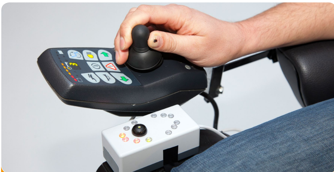
Device for safe navigation mounted on a Dupont Medical powered wheelchair
