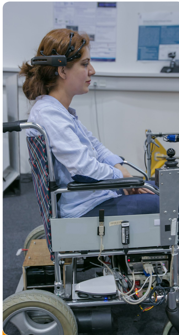
Bi-modal (EMG and Facial) human-machine interface for hands-free control of a wheelchair
